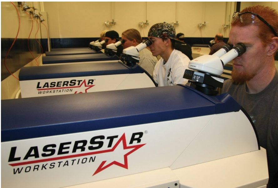
Fig. 2 — Welding students micro-laser weld aluminum joints.
