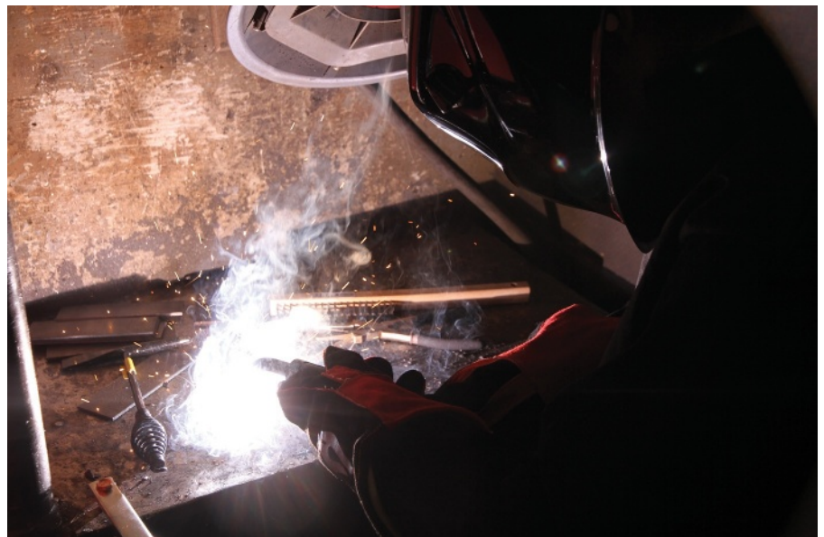
A Boy Scout completes his Welding Merit Badge using flux cored arc welding.
