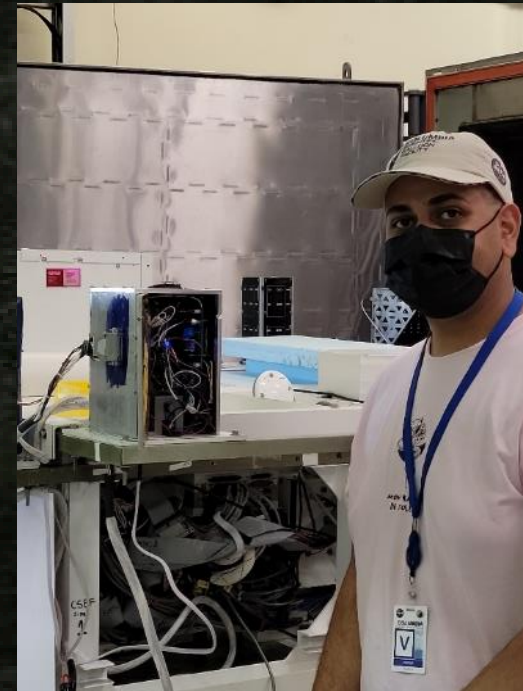
Michael integrating our payload onto the HASP platform, ready for all day thermal/vacuum testing.
