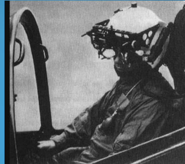
1979 - McDonnell-Douglas Corporation integrated VR into its HMD, the VITAL helmet, for military use.
