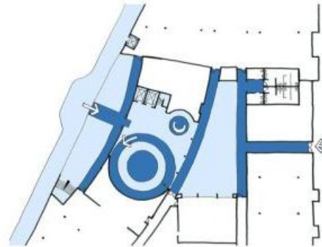
Textured Pavement Way Finding
